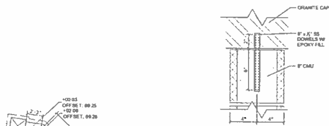
BRICK MASONRY PIN DETAIL SCALE: 1/2" = 1'-0"
