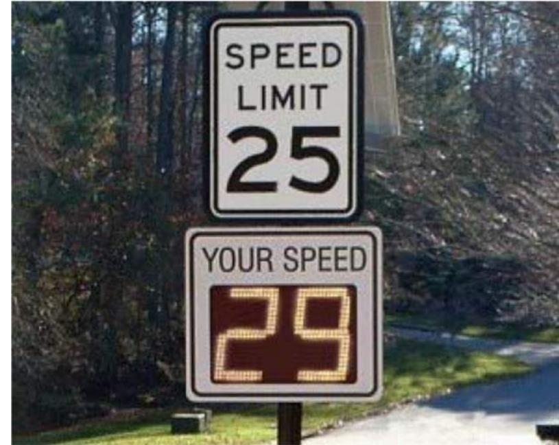
1. Speed limit signs with embedded radar
