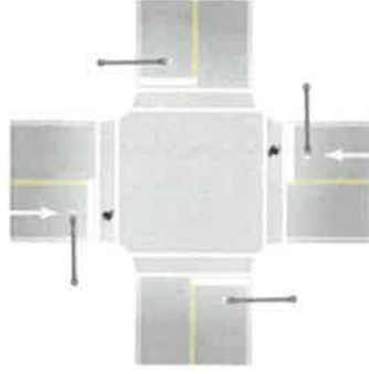
Preferred Design for Intersection Lighting Layout for Crosswalks
