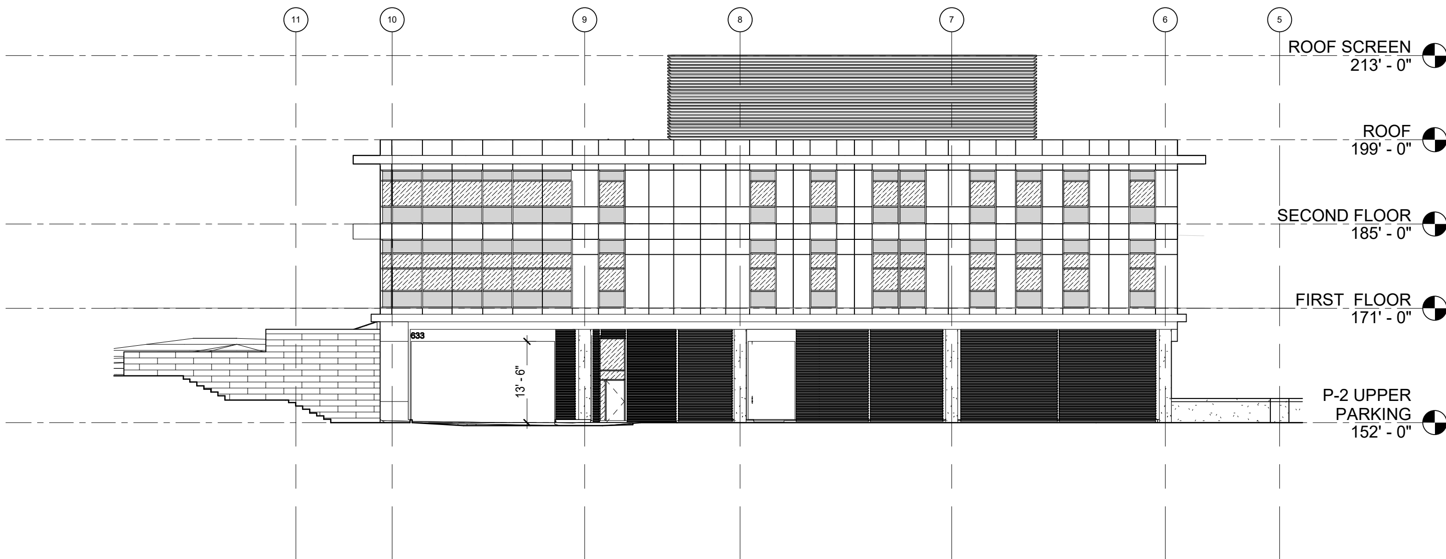
34 CROSS STREET (NORTH EAST) ELEVATION SCALE: 1/16" = 1'-0"
